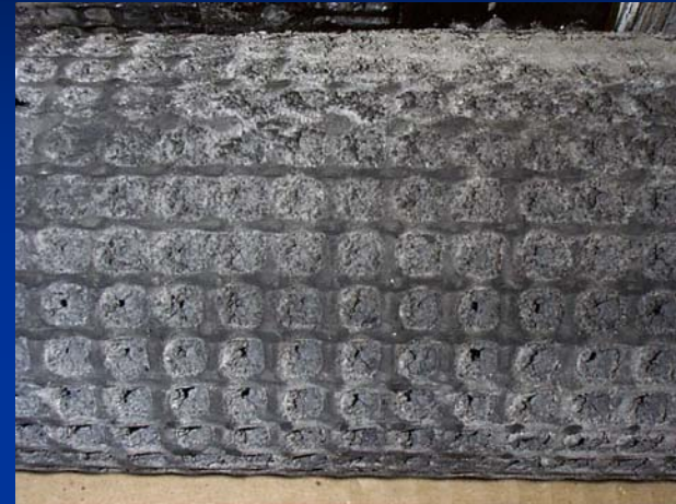
Paint Build-Up on OD of Membrane Shell.
